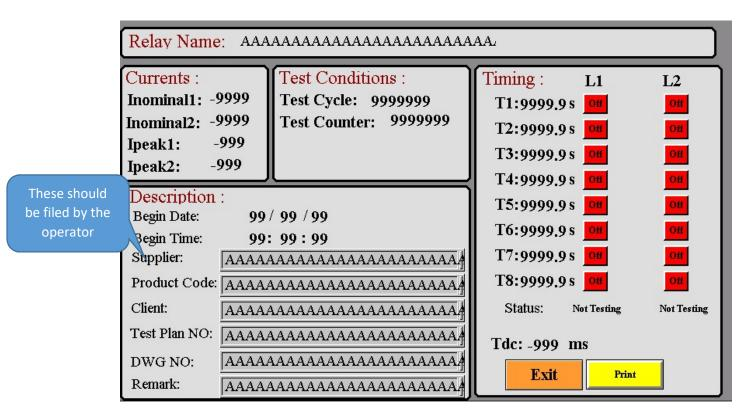
Finishing the test an alarm, showing the end of the test, will run off. Pushing the stop button, the REPORT button will appear. Energizing it the report page will pop out and you can print the report; as it was tolled before.
