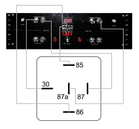
Wiring of the SPDT relays for CHANGE OVER testing
