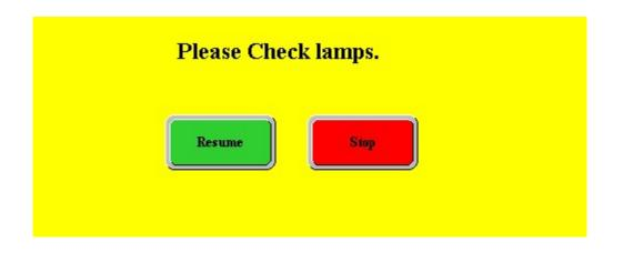
Facing the above prompt, operator has to push the Resume button. All functional lamps in the recent test will become turned on for 30 seconds. Now operator has the chance to recognize the burned lamp and change it.
